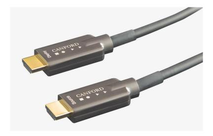
Active, optical, HDMI 2.0 cables intended for deployable applications where longer cable lengths than those obtainable with standard copper HDMI cables are required, (typically 10 - 15m max). They are also useful where the cable needs to pass through environments with high electrical interference. They offer a considerably more elegant and cost-effective solution for long cable runs than Cat5E cable with converter box systems.
