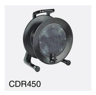
Black durable cable-drum with synthetic rubber drum and moulded high-strength plastic frame. Friction drum-brake incorporated into the frame to prevent movement in transit. Removable plastic blanking-plate over the hub, which can be punched to accept connectors as required, or removed for access to the inner tail of the cable. Folding winding-handle on the drum flange.
