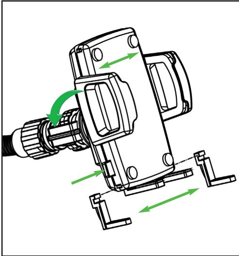
The support brackets are pushed sideways from the smartphone holder. Select the most suitable support brackets and slide it into the groove provided.
