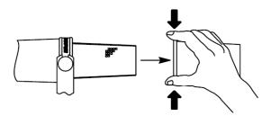
To avoid tearing the existing windshield during removal, grip from the plastic ring and the base. Remove by gently pulling and twisting.
